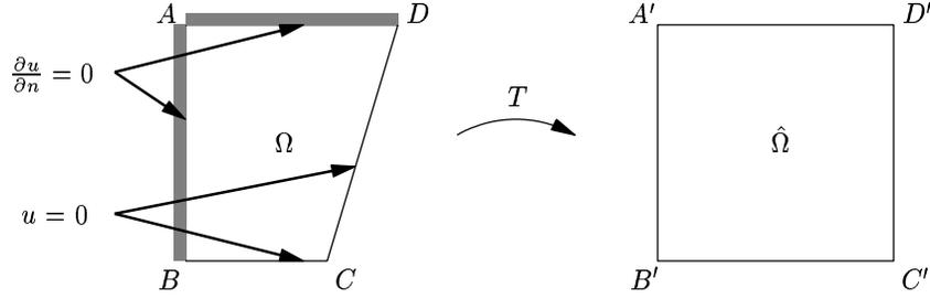
Figure 3: Geometrical transformation from the physical space to the computational domain.
