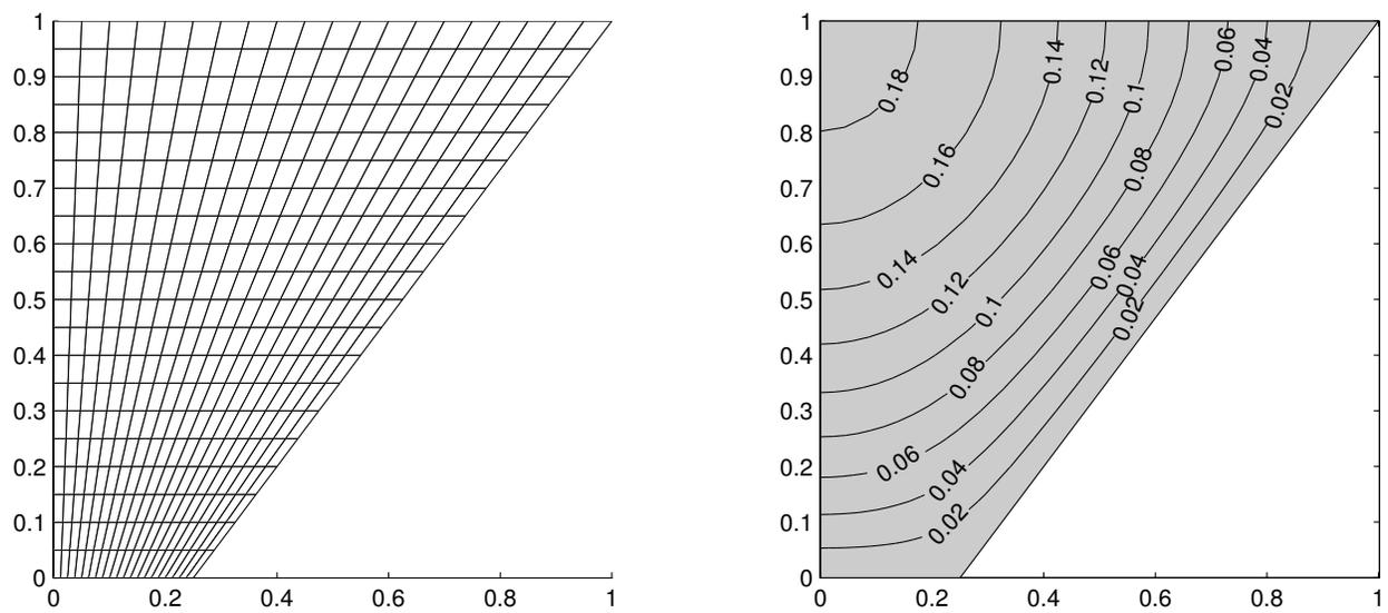
Figure 4: Sample solution, for  $l = 3.0$ ,  $b = 0.5$ ,  $h = 1.0$ , and  $N = 21$ . The plots show the grid (left) and contour lines of the solution (right). For these values, the flowrate  $\hat{Q} = 0.0574$ .
