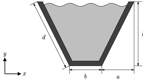
Figure 1: Trapezoidal cross section.
