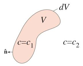
Figure 1: Schematic example of piecewise-constant coefficients  $c(\mathbf{x})$ :  $c(\mathbf{x}) = c_1$  in some region V (with boundary dV, and  $\hat{\mathbf{n}}$  denoting the outward unit-normal vector), and  $c(\mathbf{x}) = c_2$  otherwise.
