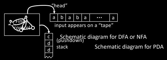
Operates like an NFA except can <u>write-add</u> or <u>read-remove</u> symbols from the top of stack.
