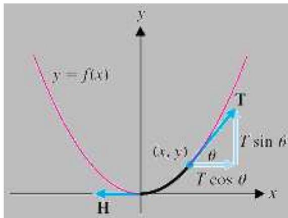
Figure 1: A hanging cable with the forces acting on it shown. From <http://www.mhhe.com/math/calc/smithminton2e/cd/folder.structure/text/chap06/section09.htm>
