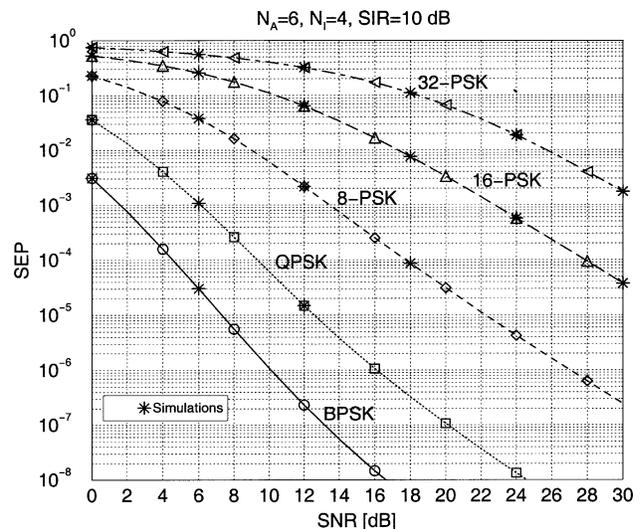
Fig. 2. SEP as a function of SNR for  $N_A = 6$ ,  $N_I = 4$ , SIR = 10 dB. Several modulation formats are considered: binary PSK, quaternary PSK, 8-PSK, 16-PSK, and 32-PSK. Semianalytical results are also provided (symbols).
