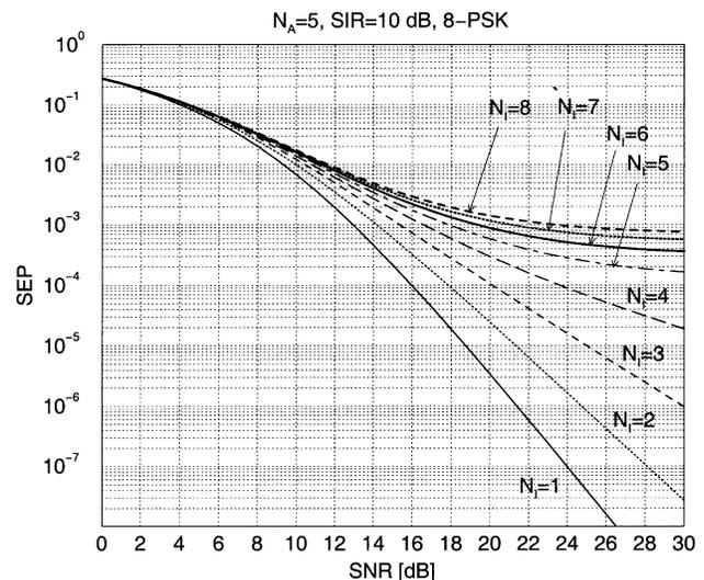
Fig. 3. SEP as a function of SNR for  $N_A = 5$ , 8-PSK, SIR = 10 dB; the number of interferers ranges from 1 to 8.
