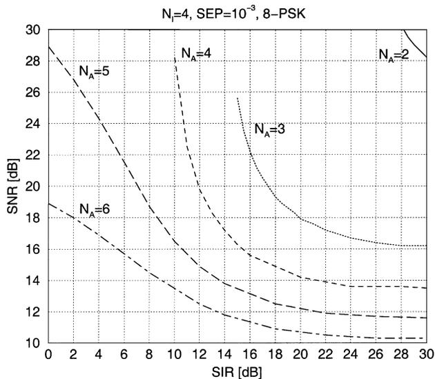
Fig. 4. SNR as a function of SIR, desired SEP =  $10^{-3}$ ,  $N_I = 4$ , 8-PSK;  $N_A$  ranges from 2 to 6.
