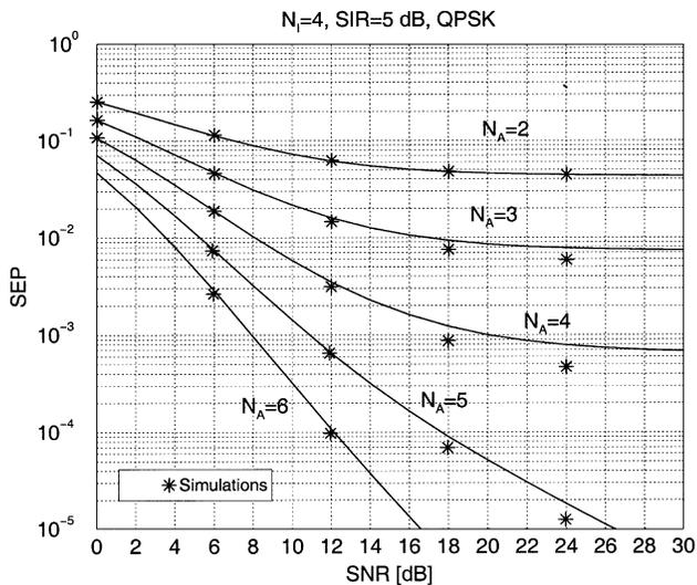
Fig. 1. Comparison between analytical and simulation results, quaternary PSK modulation,  $N_I = 4$  interferers.
