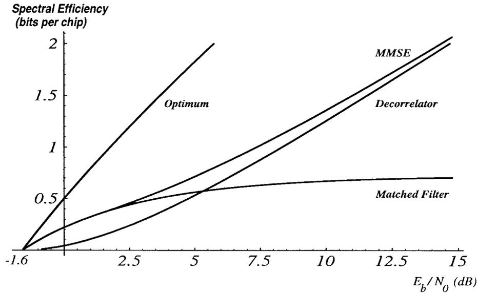
Fig. 2. Large- $K$  spectral efficiencies with optimum  $K/N$ .
