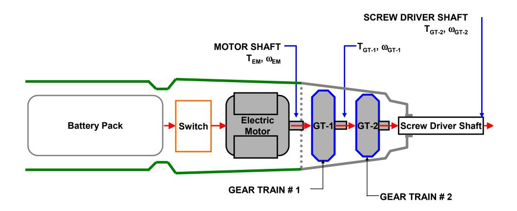
Cross Section of **Power** Flow Through Cordless Screw Driver
