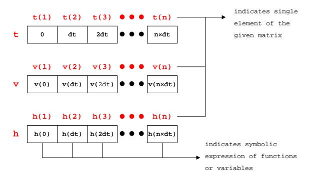
Fifth, we define the index variable to indicate current position in the matrices. It is used for indicating the relative position to current position, or for moving current position to calculate next height of the ball bouncing.
