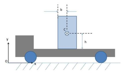
a) Find the maximum horizontal acceleration of the cart that does not cause the box to slip nor tip.
