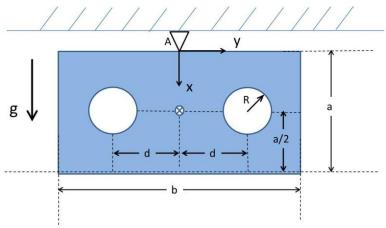
A pendulum consists of a rectangular plate (of thickness t) made of a material of density  $\rho$ , with two identical circular holes (of radius R). The pivot is at A.
