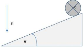
a) If the coefficients of static and kinetic friction between the wheel and the plane are  $\mu_s = 0.2$  and  $\mu_k = 0.15$  respectively, determine the maximum angle, g, of the inclined plane so that the wheel rolls without slipping.
