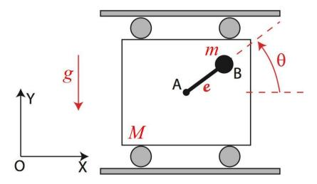
In Problem Set 3 we found the forces that the arm must exert on the mass, m, to cause it to move in a circular path about point A. These forces may be expressed as:
