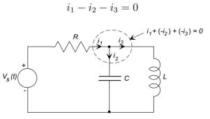
We will define a junction as a *node*, and if there are n circuit branches attached to a node
