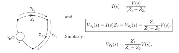
The voltage divider relationship may be used to find the transfer function of many simple systems.
