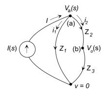
Let  $Z_1 = 1/sC$ ,  $Z_2 = R$ , and  $Z_3 = sL$ . We will use  $V_o(s) = I_2(s)Z_3$  (at node (b)), and find  $I_2(s)$  from the current division at node (a):
