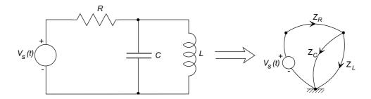
The impedance graph is shown on the right. The nodes on the graph represent *points of distinct voltage* in the circuit.
