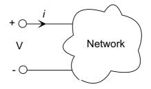
Define the *impedance* of an element or passive circuit as a *transfer function* relating current I(s) to voltage V(s) at its terminals:
