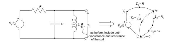
Reduce the impedance graph to a series connection of two elements
