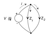
$v_{Z_1} = v_{Z_2} = V_s$
