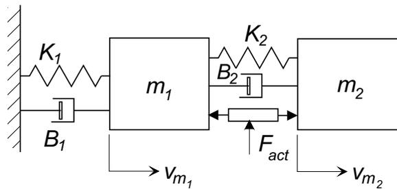
(a) In Problem Set 8 you were asked to derive the transfer function relating the velocity of the building  $v_{m_1}$  to the actuator force  $F_{act}$ . You will probably find it useful to have the transfer function relating the relative velocity  $v_{rel} = v_{m_1} - v_{m_2}$  between the building and the sliding mass. So do it ...
