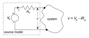
One way to do this is to model the real source(the battery) as an ideal voltage source  $V_s$  in series with a resistor  $R_o$  (the value of which is found experimentally). The voltage drop  $v_{R_o} = iR_o$  across the resistor accounts for the "droop" in the source characteristic.
