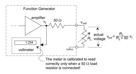
In the lab we have  $50\Omega$  terminator resistors connected across the output terminals so that the voltage reads correctly.
