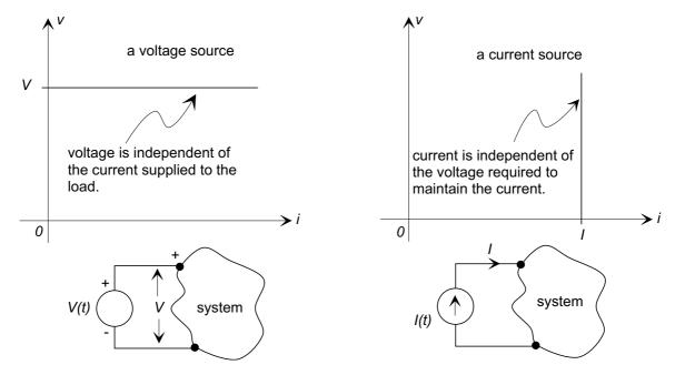
However, practical (real) sources do not have an ideal characteristic – they are power limited. For example we may think of a battery as an ideal voltage source - say with a 9 volt output, but if we were to measure the terminal voltage under increasing load currents
