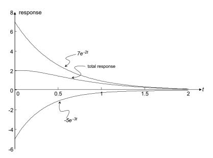
Notice that this system is stable, that is all exponential components in the homogeneous response decay to zero as time t increases.
