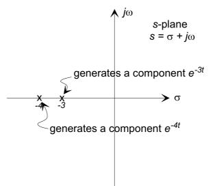
The homogeneous response components are therefore  $y_1(t) = C_1 e^{-3t}$  and  $y_2(t) = C_2 e^{-4t}$ , where  $C_1$  and  $C_2$  are defined by the initial conditions.
