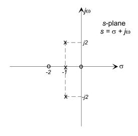
and the modal components are (1)  $Ce^{-t}$  (corresponding to the pole at s = -1), and (2)  $Ae^{-t}\sin(2t + \phi)$  (corresponding to the complex conjugate pole pair at  $s = -1 \pm j2$ ), and where the constants C, A, and  $\phi$  are determined from the initial conditions.
