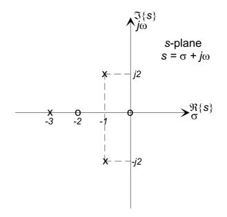
where the pole positions are denoted by an **x**, and the zeros are drawn as an **0**. The figure shows zeros at s = 0, -2, and poles at  $s = -3, -1 \pm j2$ .
