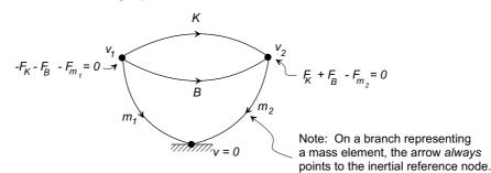
Notice the arrow directions on the branches - as implied by the right hand figure above. The graph implies a pair of continuity equations at the two nodes:
