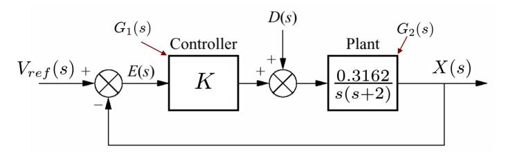
DC motor with rack-pinion load, position feedback,
