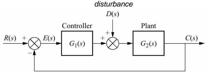
$$e(\infty) = \lim_{s \to 0} sE(s) = \lim_{s \to 0} s\left[R(s)\frac{1}{1 + G_1(s)G_2(s)} - D(s)\frac{G_2(s)}{1 + G_1(s)G_2(s)}\right] \equiv e_R(\infty) + e_D(\infty),$$
