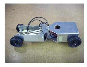
graphics, a process by which solenoid actuated valves can be used to drive the rear wheel clockwise and therefore propel the vehicle forward. What specifically is the sequence of "firing" of the pneumatic actuators you propose for propelling the vehicle?
