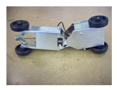
a. Make a free body diagram of the vehicle and its front and rear segements. Assume the car was proceeding straight when, at that moment, a torque of 0.3 N\*m is applied by the servo.
