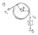
⇒ use  $\mu_s$  since tope is not moving, is static  $T_i = 5e^{0.5\frac{11}{16}\pi} = 2.81 \text{ M} \Rightarrow 10 \text{ Keep Frank dipping down}$   $T_i = 5e^{0.5\frac{11}{16}\pi} = 8.89 \text{ M} \Rightarrow 10 \text{ Keep Frank politing too}$ For back
