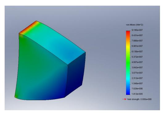
This is just a very rough approximation, since the load won't be evenly distributed and SolidWorks doesn't even have a Delrin model. But it shows a maximum stress of 92MPa at the tooth base. This is greater than the yield stress of Delrin. The factor of safety in this case would be below one, meaning the gear is likely to fail. Your exact calculation will depend on your gear train design, but many would likely fail under the stall torque of the servo.
