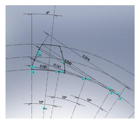
If you showed this construction, using arc lengths to generate the shape from the base circle, either in SolidWorks or by hand, that was worth full credit. Simple extruding the provided drawing into a 3D part was not the intent of part a), but given the server issues substantial credit will be given for just about anything that looks like a 24-tooth gear.
