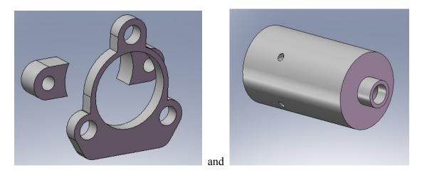
The procedure includes milling the flat pieces and turning/facing/drilling/boring the cylindrical piece, then assembling them by various means. Cutting the flat pieces on the water jet is an option, but you will have some taper on the edges.
