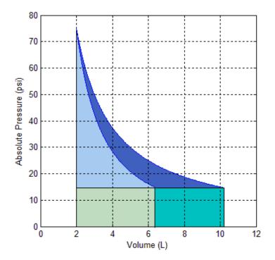
This shows the relevant integral components for both 3a and 3d. The adiabatic curve does less work than the isothermal curve puts in, as expected. The efficiency in this case is about 60%.
