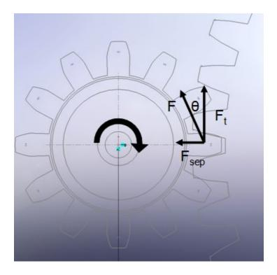
The true force between the gears acts along the pressure line. The tangential force is one component of this true force. The separation force is the other component. Then, the calculation of the separation force goes like:
