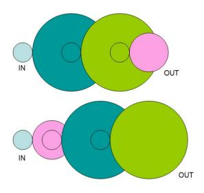
The latter is probably easier to build since all the gears can be supported by bearings on both sides. (The final output gear of the former cannot.) There are obviously many more ways of arranging this.
