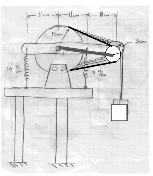
Due to the small angles and generous  $\pm$  20% allowance for our estimate, we can linearize. We have a motion of the weight due to two factors: Rotation of the arm => 0.1 rad\*24\*cm=2.4 cm downward
