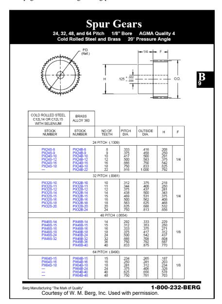
C) (5 points) If gear PX24B-8 and PX24B-22 are mated together 0.02 inches farther apart than you determined in part A, what are the primary consequences? Would your answer to part B change and if so would it rise or fall?
