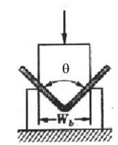
Figure 2: sketch of V-die bending
