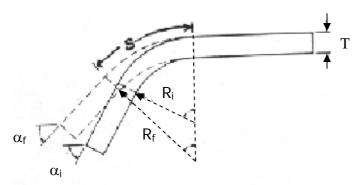
Figure 1: schematic of springback bending
