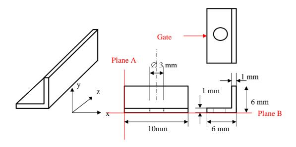
Figure 1: L-bracket part drawings
