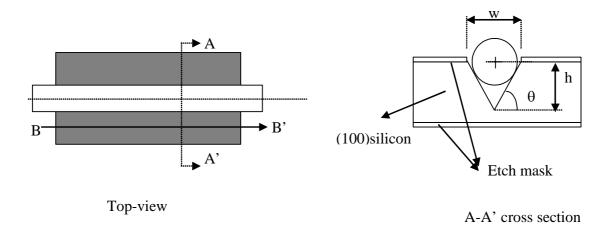
Figure 2-1 A self terminated V-groove is formed on the {100} plane.
