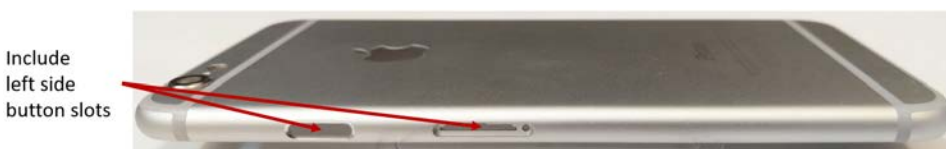
Figure 4: Include left side button slots in the process plan.
