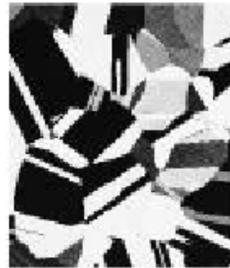
10 min at 700 C: grain growth
