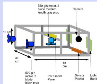
**Original Vehicle Design:** This design is different than our final design in that our final design has no instrument panel, has the back motors attached differently, and has the sensor packet above the motor.
