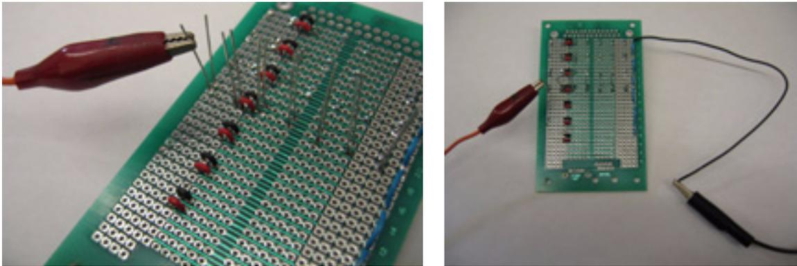
**Figure 10: Testing the First LED Row. Positive Lead (right) and Negative Lead (left)**
