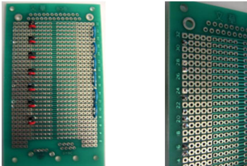
**Figure 7: Protoboard with Row Connection Wires: Front (left) and Back (right)**
