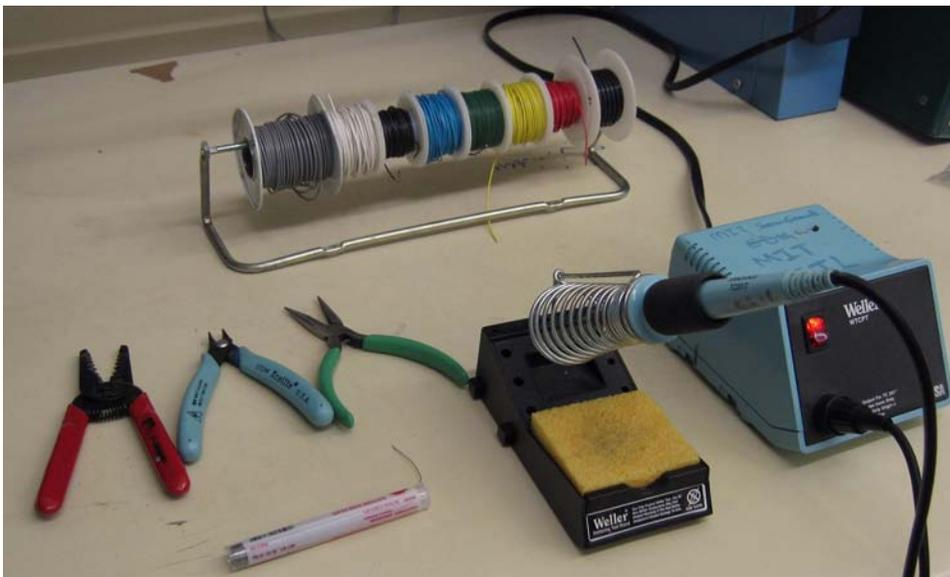
**Figure 3: Tools for Building LED Light Bank**
