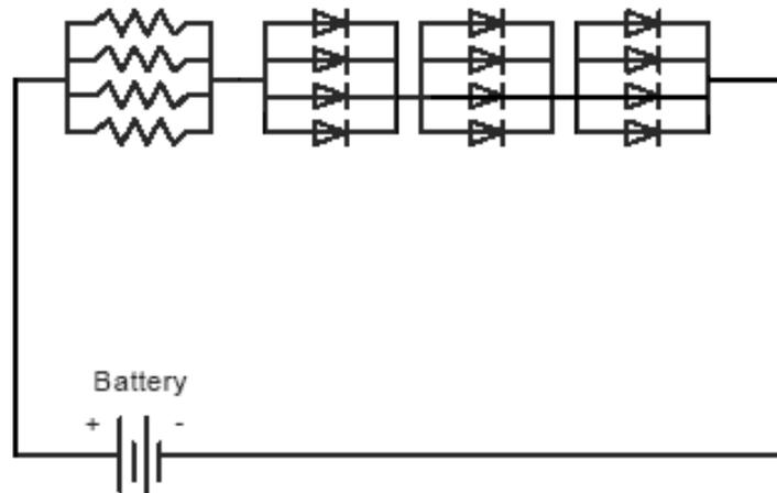
**Figure 2: Circuit Diagram for LED Light Bank**
