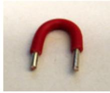
**Figure 5: Bent Jump Wire**
