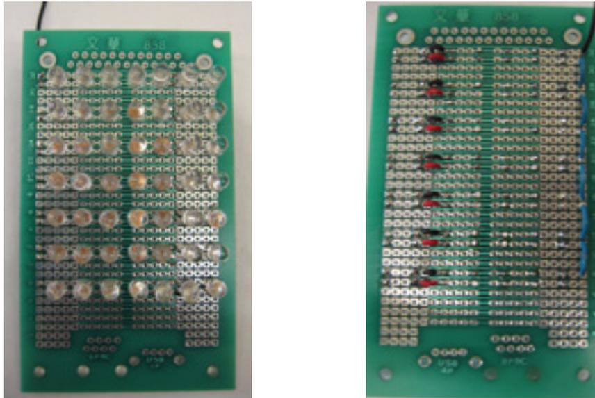
**Figure 11: All Rows of LEDs: Back (Left) and Front (Right)**
