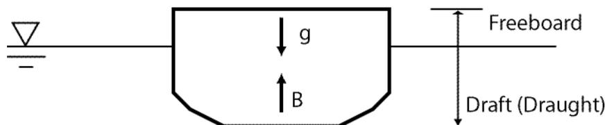
*A vessel in static equilibrium with the centers of gravity*
