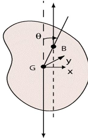
We can write the equation of motion in terms of the rotational displacement,  $\theta$ , and rotational acceleration,  $\ddot{\theta}$ :
