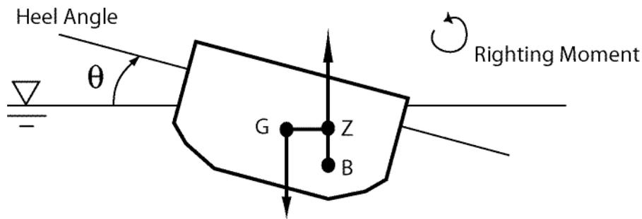
*A statically stable vessel with a positive righting arm.*
