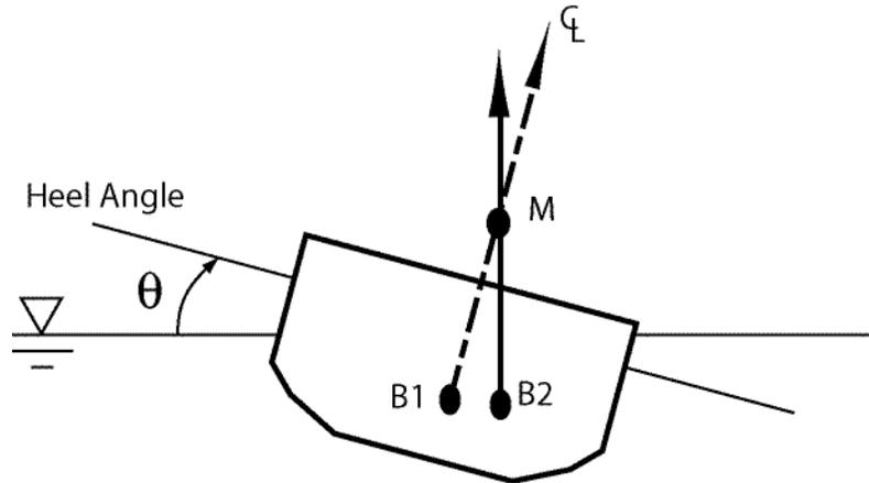
*The metacenter is the intersection of two distinct lines of action of the buoyancy force.*
