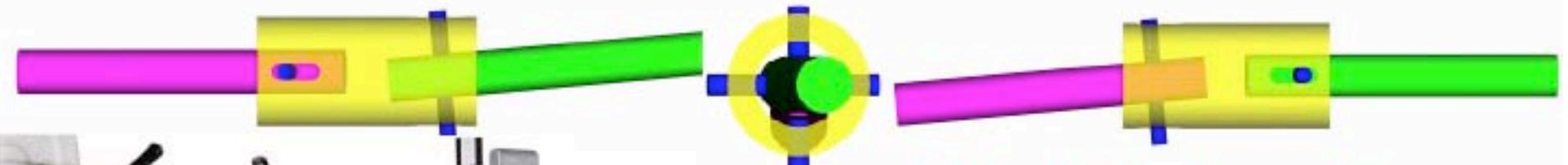
*Critical: Note the clearance between the coupling bore and both shafts!*
