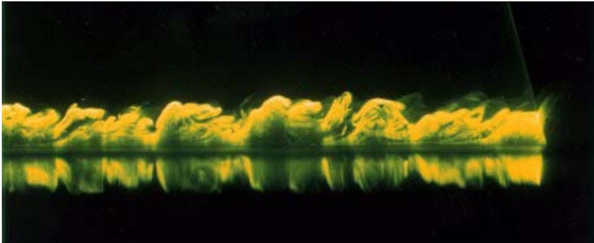
This picture is a side view of the large eddies in a turbulent boundary layer. Laser-induced fluorescence is again used to capture the quasi-periodic coherent structures. Flow is from left to right.
