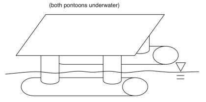
The diameter of the uprights is 10 m, and that of the pontoons is 10 m. The length of the pontoons is 100 m. The added mass of the uprights is negligible compared to that of the pontoons.
