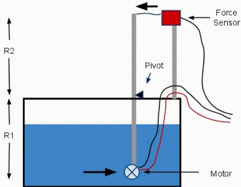
$$\text{Force} = \text{Sensor Force} \times R2/R1$$
