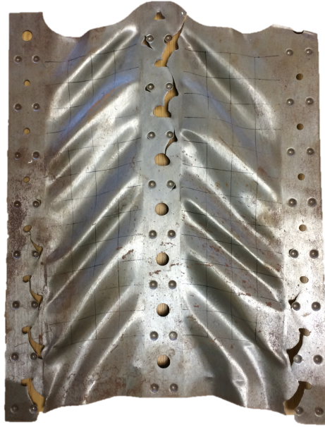
Figure 11.8: A photograph of shear buckling of a plate representing the damage pattern on the ship's hull inflicted upon grounding.
