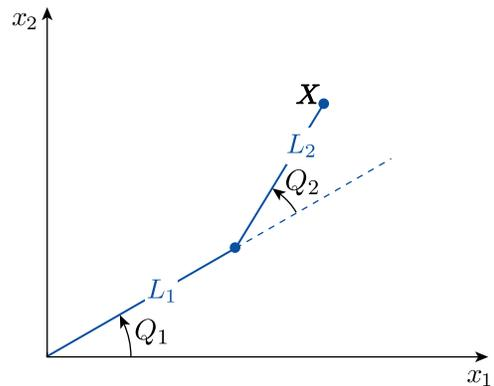
Figure 2: Schematic of robot arm: end effector  $\mathbf{X} = (X_1 \ X_2)^T$  and joint angles  $\mathbf{Q} = (Q_1 \ Q_2)^T$ .
