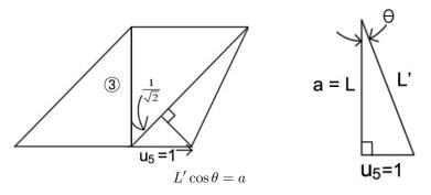
We use the approximations  $\cos \theta = 1$ ,  $\sin \theta = \theta$  because the displacements are small, and we are performing an infinitesimal displacement analysis. So, L' = a.
