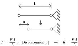
Truss bars can only resist axial forces. Note that the length of bar 3 does not change in infinitesimal displacement analysis!
