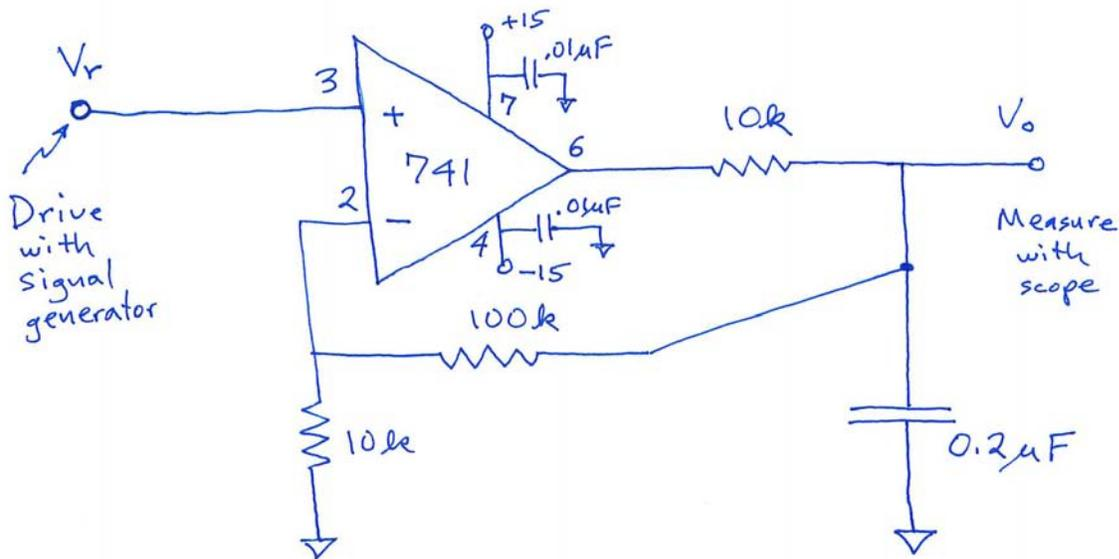
Build this circuit on the protoboard of your myDAQ kit. Be sure to connect power to the op amp and use the indicated bypass capacitors. For this circuit:
