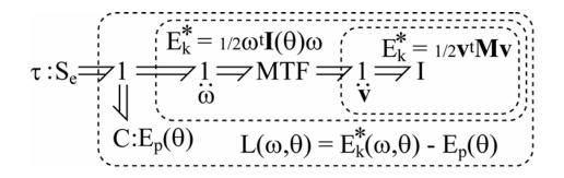
Mechanism in "uncoupled" inertial coordinates: (innermost box in the figure)
