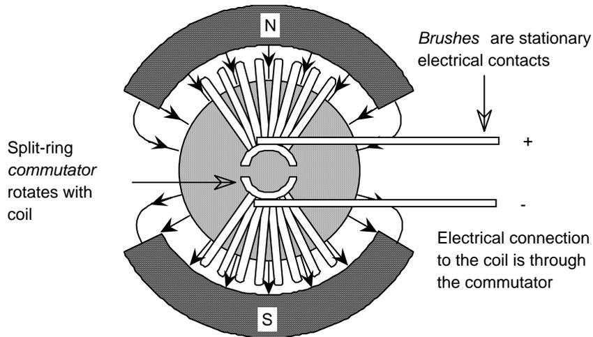
Figure 6: Schematic of the mechanical commutation system used in a direct-current permanent magnet motor.
