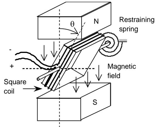
Figure 3: Conceptual sketch of a D'Arsonval galvanometer.
