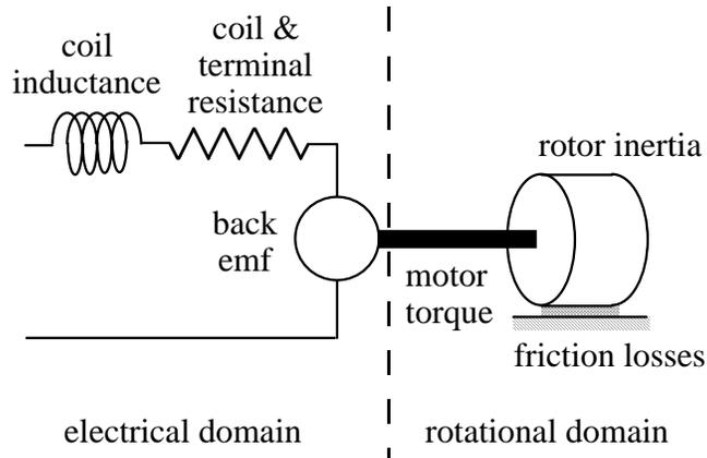
Figure 7: Schematic diagram of a DCPMM model with “parasitic” dynamics
