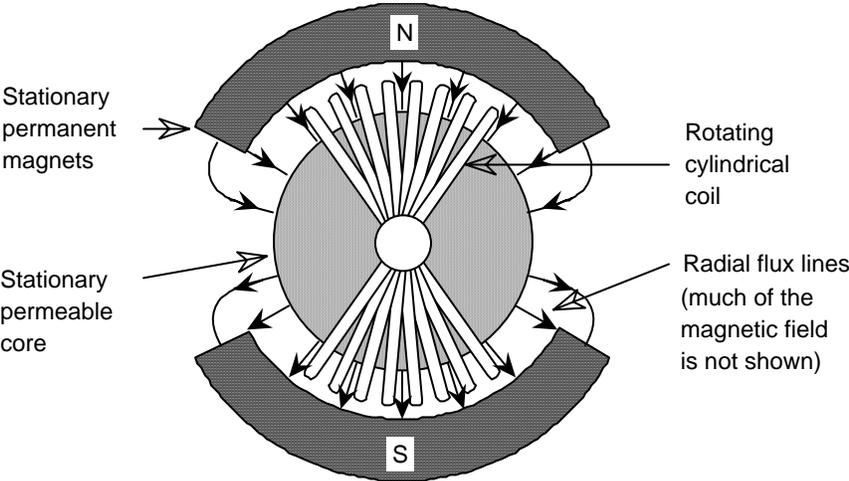
Figure 4: Schematic end-view of a D'Arsonval galvanometer modified to reduce the angle-dependence of the transduction equations.
