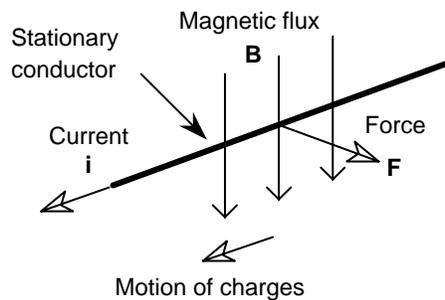
Figure 1: Forces on a current-carrying conductor in a magnetic field.
