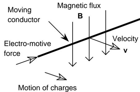
Figure 2: Voltage across a conductor moving in a magnetic field.
