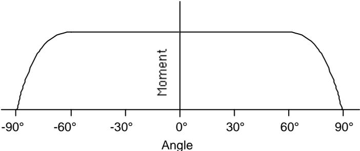
Figure 5: Sketch of half of the constant-current torque/angle relation resulting from the design of figure 4.
