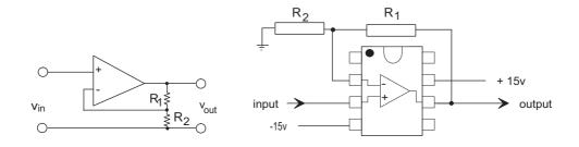
In this case  $R_1$  and  $R_2$  act as a voltage divider, and
