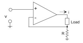
Assume that the op-amp drives a load of unknown resistance. A small resistor R is placed in series with the load. Then the inverting input is  $v_{-} = iR$ . At the output of the amplifier
