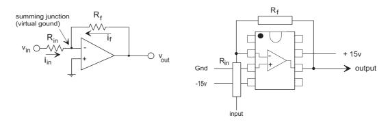
The non-inverting input is connected to ground and a pair of resistors,  $R_{in}$  and  $R_f$  (the feedback resistor) is used to define the gain. To simplify the analysis we make the following assumptions:
