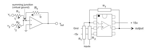
As before we assume that the inverting input is at a virtual ground  $(v_{-} \approx 0)$  and apply Kirchoff's current law at the summing junction
