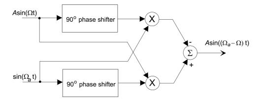
A  $\pi/2$  phase-shifter is easy to build for a single frequency, such as  $\sin(\Omega_a t)$  but when the input signal, such as a speech signal, contains more than just a single component each spectral component must be shifted by 90°. This requires an all-pass filter with a constant phase shift, which is a difficult design task for a continuous filter. Approximations as active or passive filters are available.
