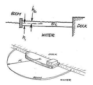
Oil Spills may occur in ports where oil tankers are loaded. The density of oil,  $\rho_o$  is less than that of water  $\rho_w$ , and the two fluids are immiscible, so that when a spill occurs the oil simply spreads out in a layer on top of the water. To contain any possible spills, a semi-circular "oil boom" is deployed at a radius R around the dock where the loading takes place.
