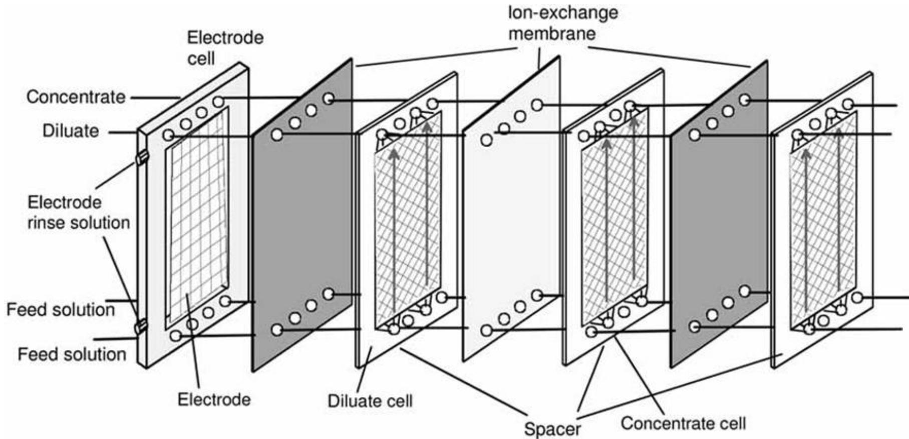
an electro dialysis stack is composed of 100 to 400 cell pairs between electrode compartments
