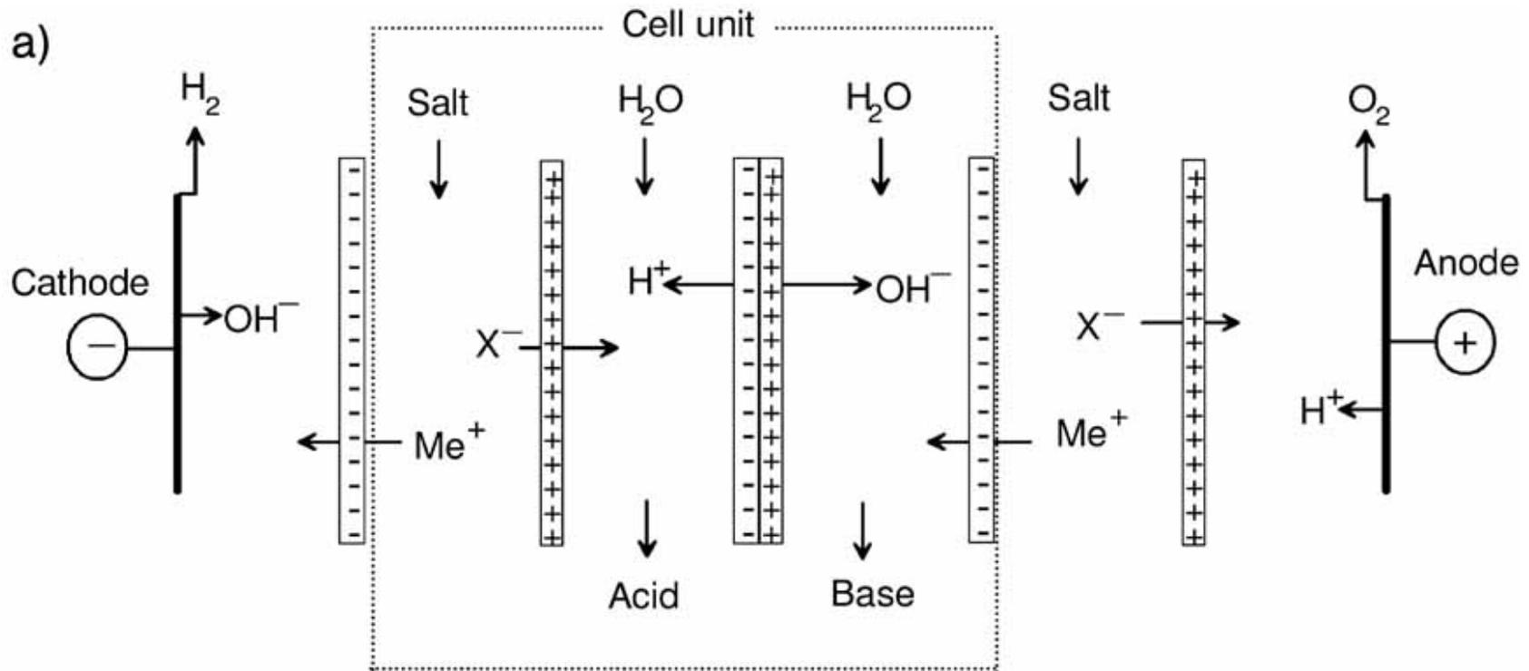
production of acids and bases from the corresponding salt solutions
