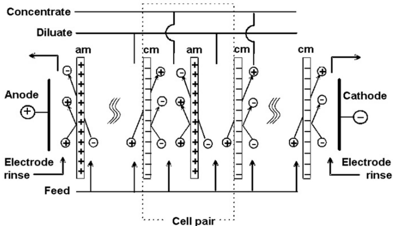
ions are removed from a feed solution and concentrated in alternating cells
