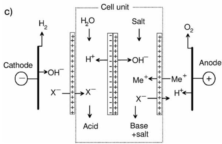
production of a pure base and an acid-salt mixture
