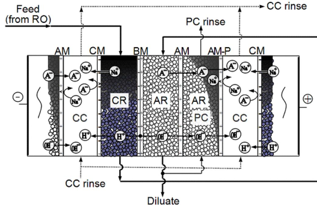
good removal of weak acids, repeating units can be stacked between electrodes, maximum achievable resistance < 10 M Ωcm
