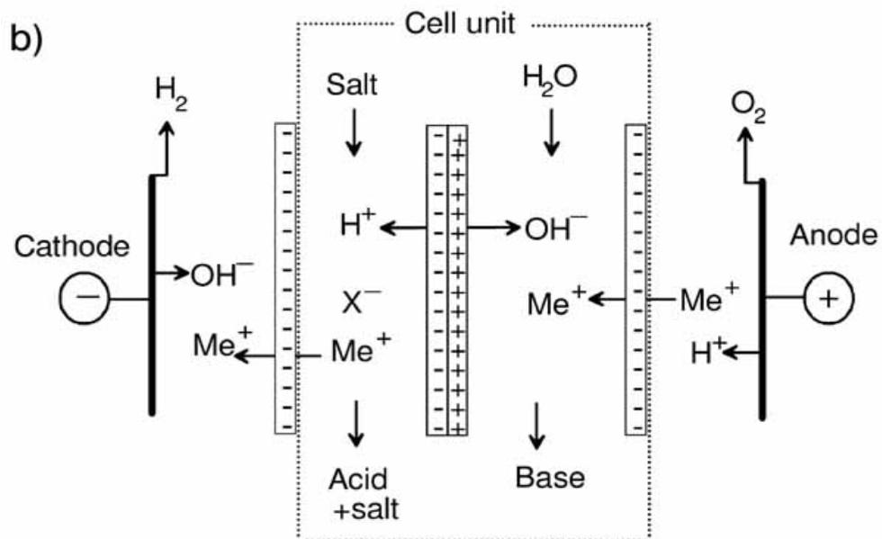
production of a pure acid and a base-salt mixture
