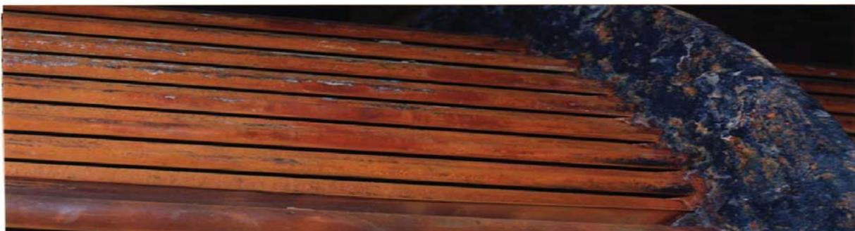
Details of tube bundle and tube support
