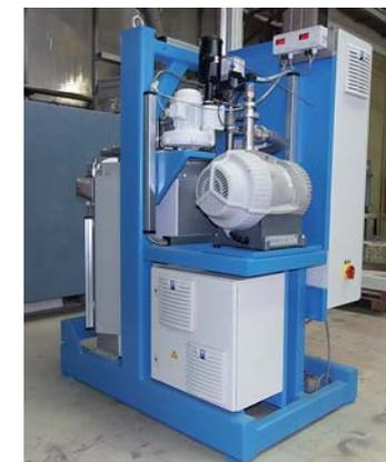
Fraunhofer Institute,  $Ba_{0.5}Sr_{0.5}Co_{0.8}Fe_{0.2}O_{3-\delta}$ , uses tubular membranes, heat recovery to achieve  $0.14 \text{ kWh}/\text{kg}_{O_2}$
