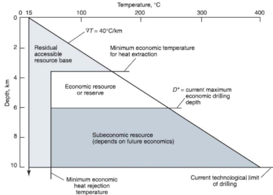
Figure 11.4. Idealized depth versus temperature profile for a hypothetical  $40^\circ\text{C}/\text{km}$  geothermal resource. The resource base and economic resource or reserve regions are shaded in different tones to illustrate the factors limiting the portion of the total resource base that can be economically produced with a specified set of technologies and economic factors. Adapted from Tester and Grigsby (1980). Reprinted with permission of John Wiley & Sons.
