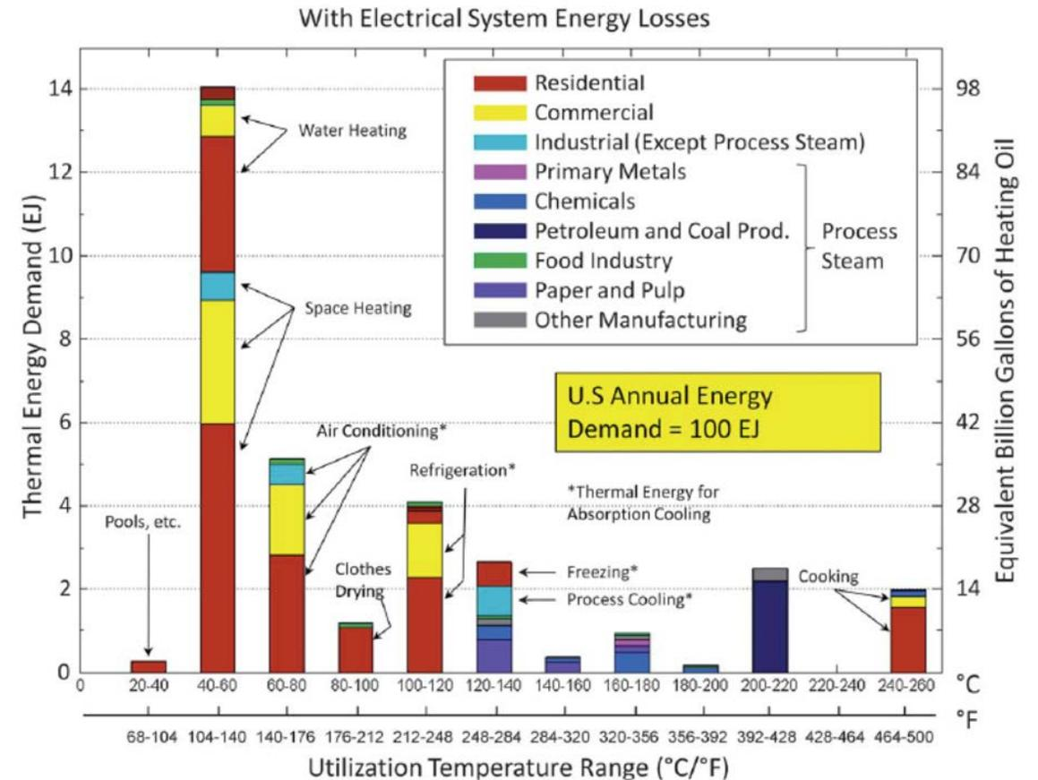
Fig. 1 Estimated thermal energy consumed in America below  $260^{\circ}\text{C}$  ( $500^{\circ}\text{F}$ ).
