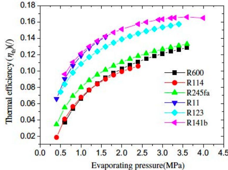
(left) The  $T$ - $s$  diagram of an ORC using a fluid with an overhang saturation curve, and (right) using a number of different working fluids. The analysis applied realistic models for the different cycle components and working fluid equation of state. The cycle operates on engine exhaust 250 °C. Results show the impact of the cycle high pressure Tian et al., *Energy*, 47, 125–136, 2012.
