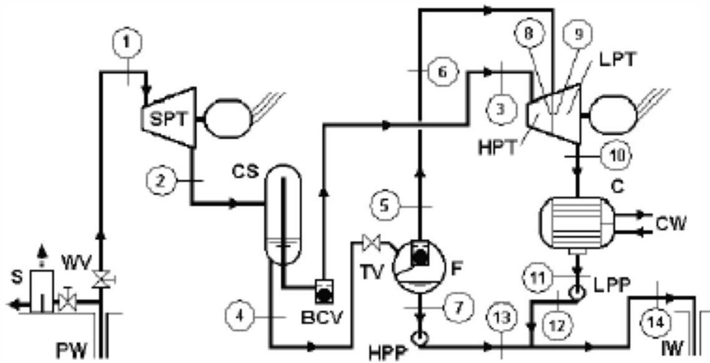
Trilateral supercritical vapor cycle
