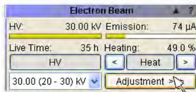
7. Select the accelerating voltage (0.5kV, 10kV and 30 kV) using combo box on the Electron Beam panel.
