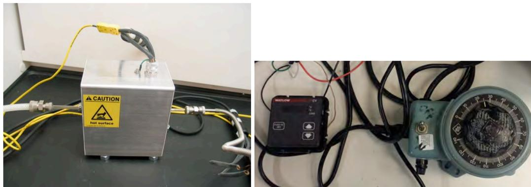
**Fig. 8 Gas pre-heater and controller**
