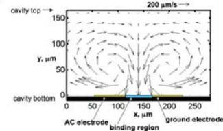
Fig. 2 Numerical model of electrothermal velocity. Two long-parallel electrodes on cavity bottom are driven at 200 kHz, 10 V<sub>pp</sub>. Maximum electrothermal velocity generated is 1.1 mm s<sup>-1</sup>, near the inside edges of the electrodes. Cavity sides extend well beyond plotted region.
