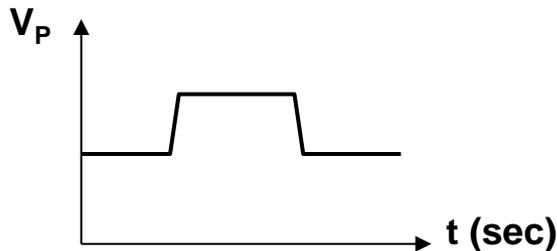
*Applied voltage to the piezo-actuator*
