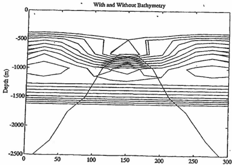
FIG 6. Interpolated profiles with and without "seamount" bathymetric feature. Interpolation is largely unaffected by presence of bathymetry, except inside the seamount where the result is meaningless anyway.
