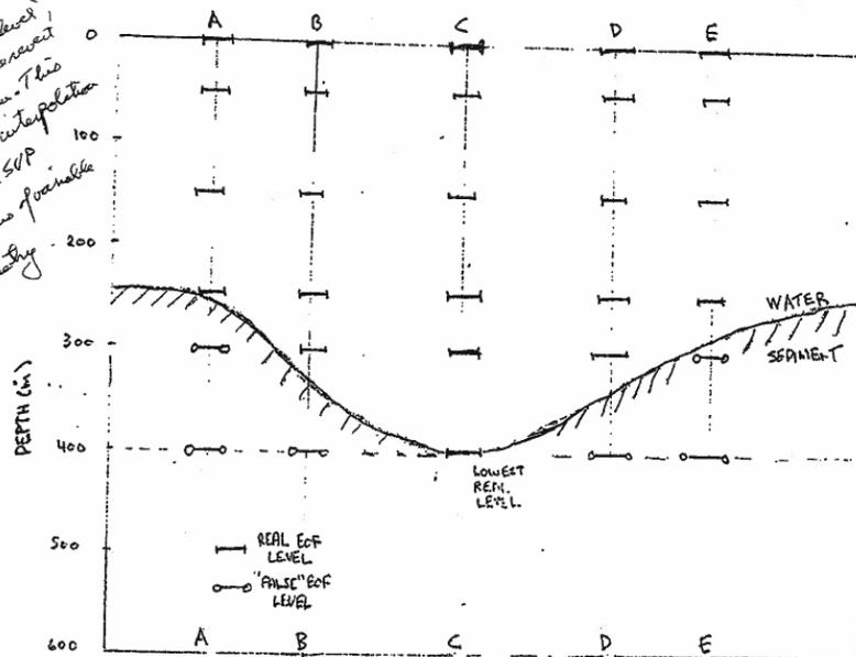
FIG 1. Variable bathymetry region EOP interpolation for water column
