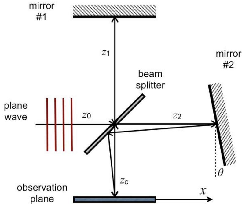
Neglecting the truncation of the plane wave due to the finite size of the optics, write an analytical expression for and sketch the interference pattern as function of coordinate  $x$  at the observation plane.
